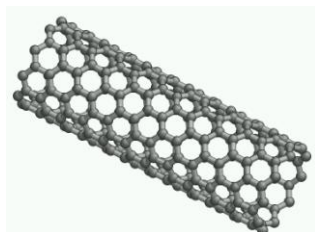
[Fig 6] – The structure of a carbon nanotube.
