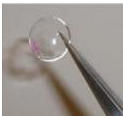
Figure 4: The chemical reaction with glucose gives a pink tinge to the lenses, alerting the patient to a change in their blood glucose levels without needing to use a finger lancet
