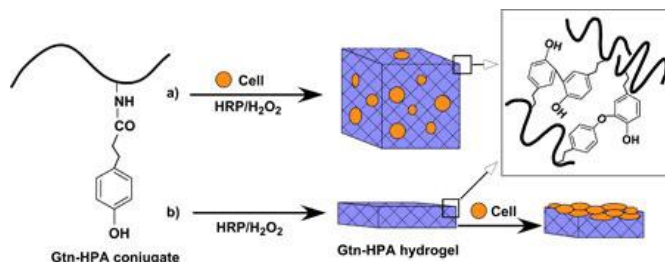
Figure 7 - formation of Hydrogels by enzyme-catalysed oxidation for (a) 3D and (b) 2D cell growth/differentiation.
